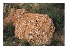
† Figure 197: Typical quartz-pebble conglomerate of the Amazon reef, as it was mined in the past on the farm Rooderand 510 IG in the Venterskroon Goldfield. The pen, for scale, is 12 cm long.
